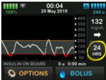
1 Hour Trend Graph shows you your current sensor glucose reading along with the last 1 hour of sensor glucose readings.
