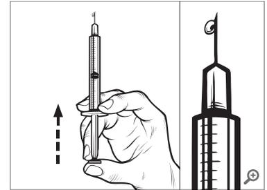
9. Re-insert the needle in the fill port and slowly fill the cartridge with insulin. It is normal to feel some
