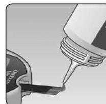
Touch and hold the hanging drop of control solution where the narrow channel meets the **TOP EDGE** of the test strip. Make sure the confirmation window fills completely. Control solution should not be applied to the flat face of the test strip.
